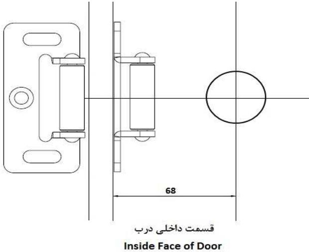
2-The distance of the door hole to the jamb is 68 mm
